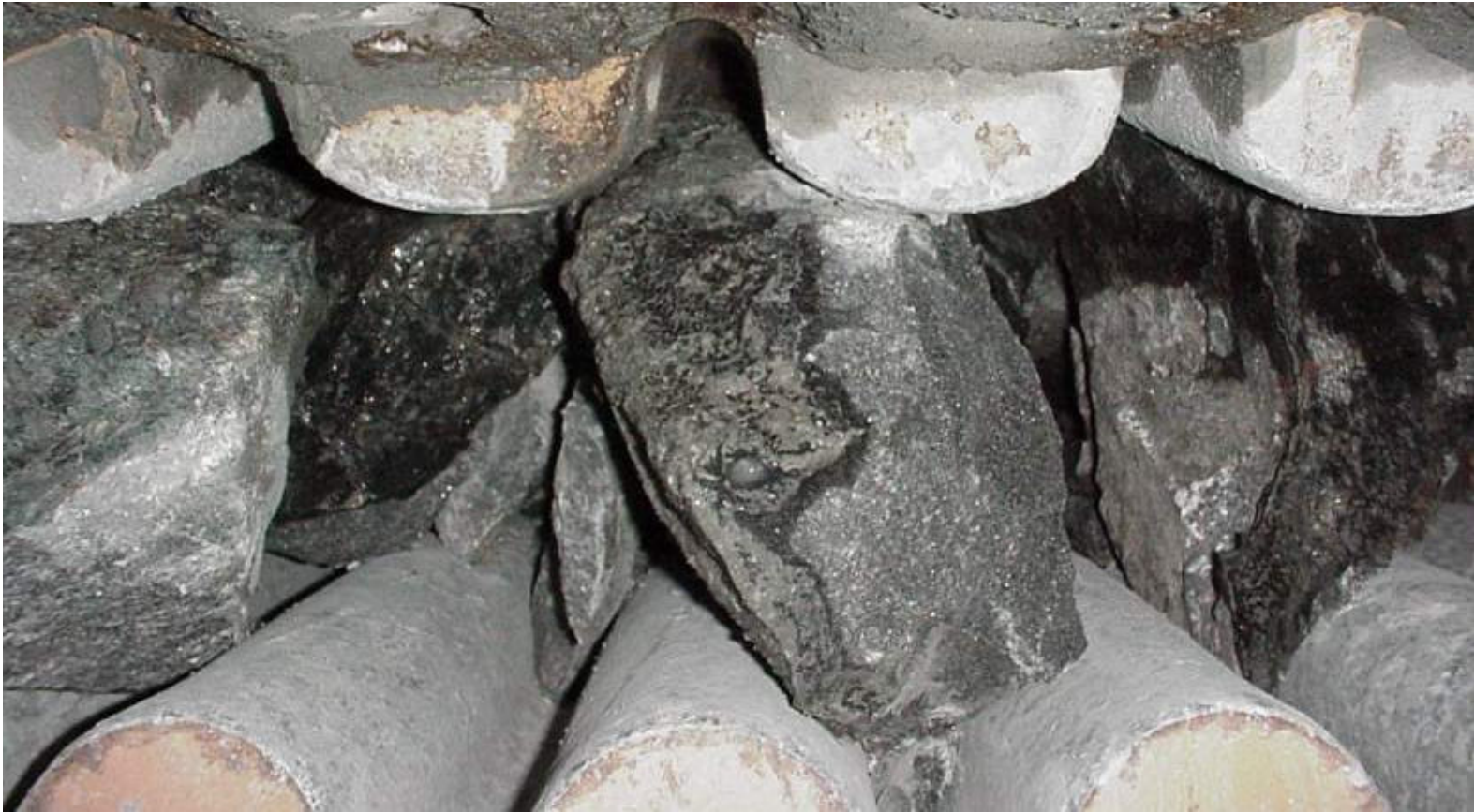
Discharge end of jaw crusher, viewed from beneath
