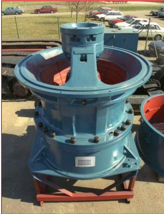
Gyratory or cone crusher
