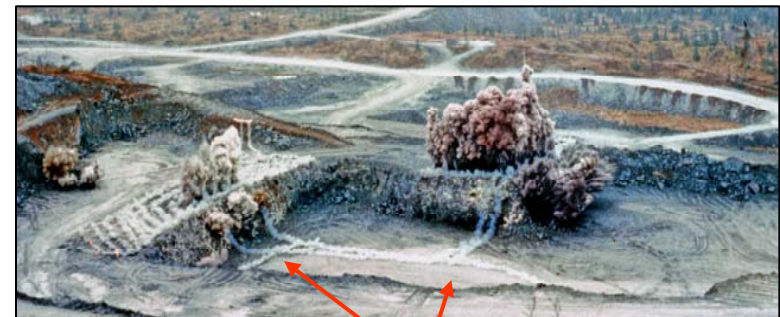
Stemming ejection and gas venting in bench walls resulting in excessive air blast and reduced heave and throw
