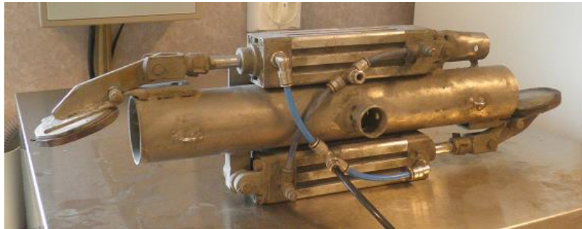
Figure 4.3: Sampling probe used in flotation cell characterization test work.
