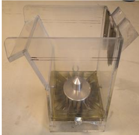
Figure 2.6: Eight litre batch flotation cell used by the Boliden mineralogical lab.
