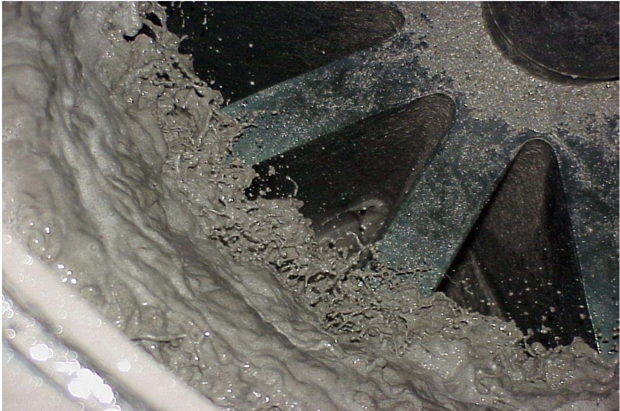
Figure 2: The interaction between air and pulp on the tip of a rotor.
