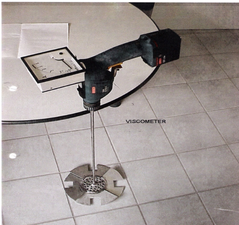
Figure 67: Showing the modification to the hand drill and design of the shear plate for the Helephi's viscometer.
